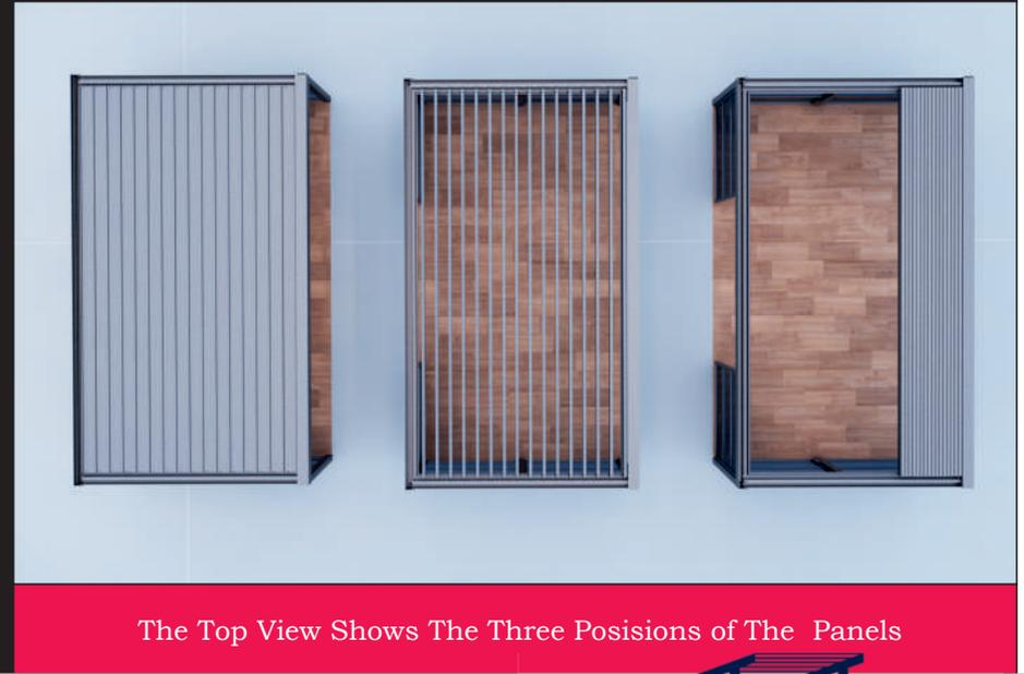
The Top View Shows The Three Positions of The Panels
